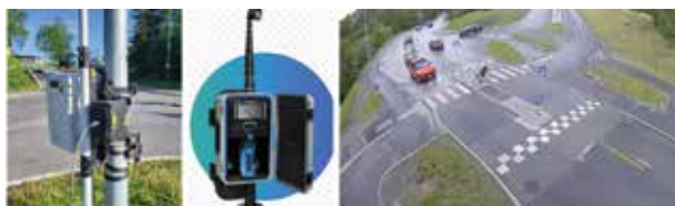
Figure 5: Both types of Scouts attached to one street light pole (left); Scout Plus unit (middle); a view captured by Scout Plus (right)
